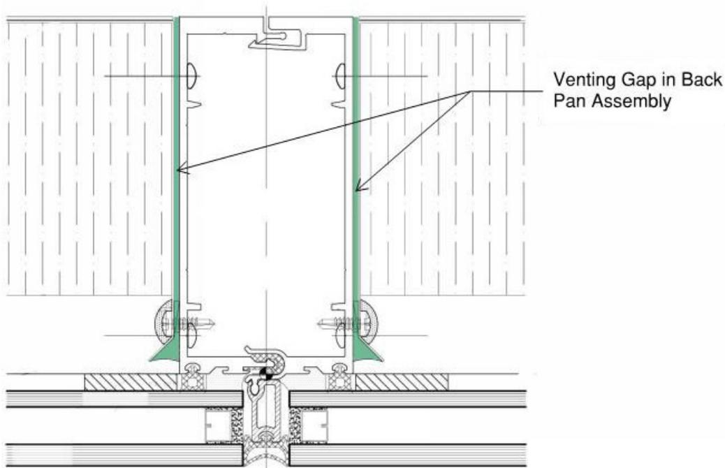
Figure 4: Shadow box ventilation to the building interior.
