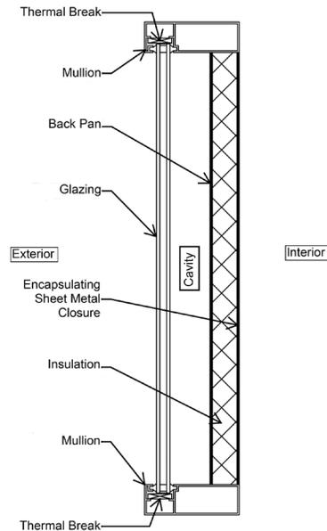
Figure 1: Components of a typical shadow box.
